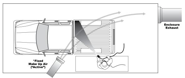
\* The volume of air supplied by this unit is dependent on the size of the enclosure exhaust unit, therefore the volume of make up air is determined on a case by case basis.
