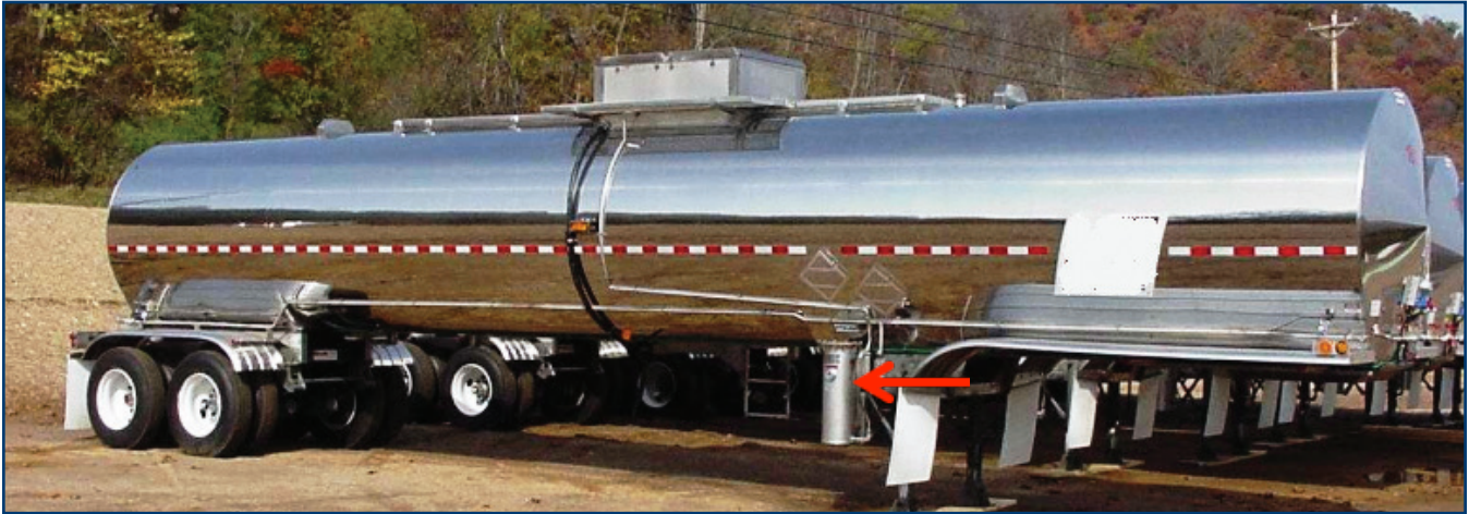
The above photo points to the desiccant dryer located on a Cargo Tank Trailer.
