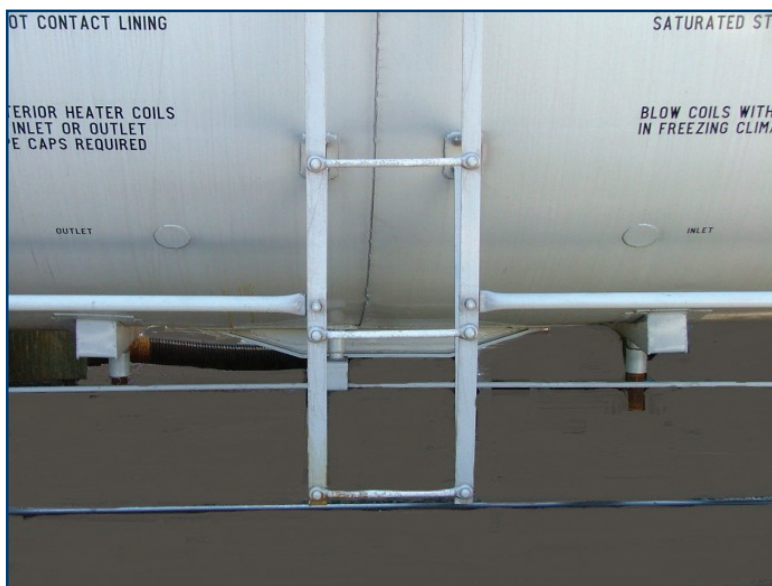
This photo illustrates the heater coil inlet and outlet on the bottom of a Rail Tank Car.
