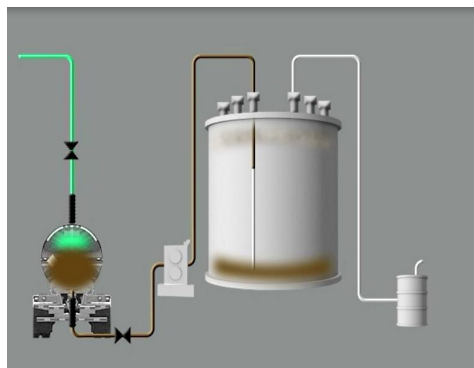
Figure 4: Cargo Tank Trailer Pump Transfer with Pressure Assist
