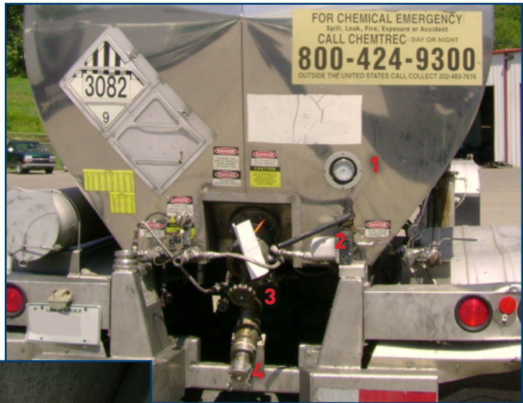
The above photo points to the desiccant dryer located on a Cargo Tank Trailer.
