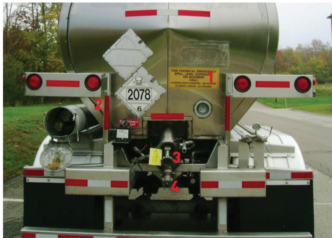
The above photo illustrates the rear unloading area of a Cargo Tank Trailer: 1) Temperature Gauge; 2) Hydraulic Jack to Operate Internal Valve; 3) External Valve; 4) 2-inch Unloading Connection.
