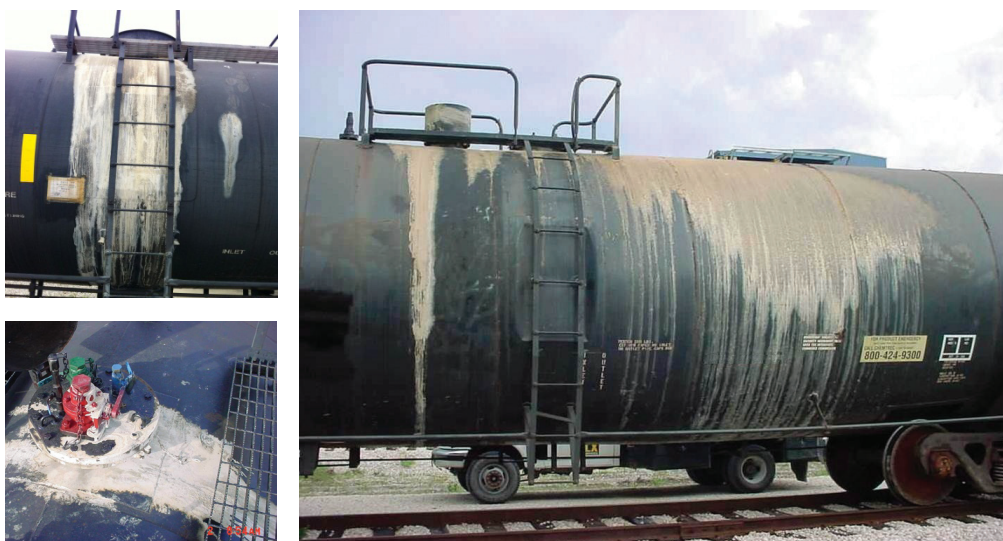
The above photos illustrate a rail car with external residue that would need to be removed prior to transport.
