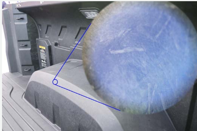
2019 GMC Sierra Denali lightweight carbon fiber composite truck bed with pocket reinforcements made from recycled carbon fiber thermoplastic materials.
