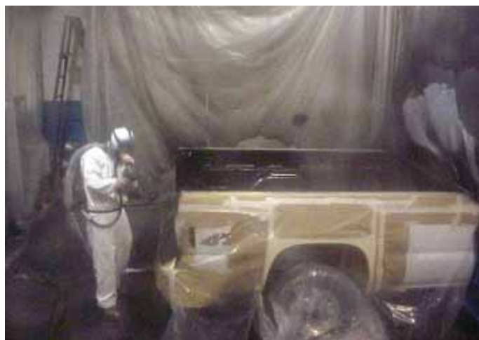
Spraying base coat with protective equipment.
