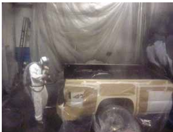
Figure 1. Spraying base coat with protective equipment.
